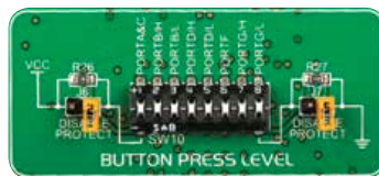
Figure 6-5: Button press level DIP switch (tri-state)
