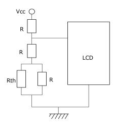
Temperature Compensation (RF circuit)
