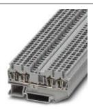
Feed-through terminal block, Connection method: Spring-cage connection, Cross section: 0.08 mm² - 4 mm², AWG: 28 - 12, Width: 5.2 mm, Color: gray, Mounting type: NS 35/7,5, NS 35/15
