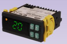
The IR33 refrigeration controllers are designed for management of refrigeration and food processing applications. The controllers have 2 NTC inputs for ambient and defrost temperatures and versions are available which have 1, 2, 3 or 4 relay outputs for control of the compressor, active defrost, evaporator ventilation fan and auxiliary output. Versions incorporating a real time clock and HACCP function are also available.
