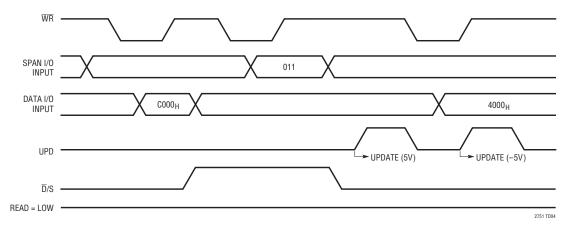
3. Write and update mid-scale code in 0V to 5V range ( $V_{OUT} = 2.5V$ ) using readback to check the contents of the input and DAC registers before updating.
