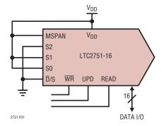
Figure 1. Configuring the LTC2751 for Single-Span Operation (±10V Range)
