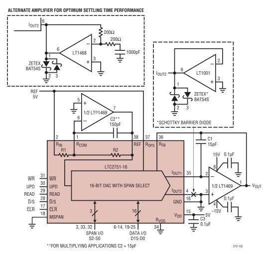
Figure 2. Basic Connections for SoftSpan  $\rm V_{OUT}$  DAC with Two Optional Circuits for Driving  $\rm I_{OUT2}$  from GND with a Force/Sense Amplifier
