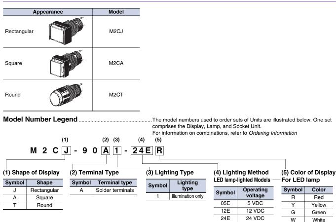
One set comprises the Display, Lamp, and Socket Unit.
