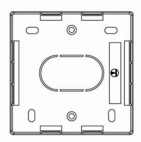
TUK:3L37b 86X86x37mm BACK BOX TOLERANCE UNLESS OTHER SPECIFIED :±0.15MM
