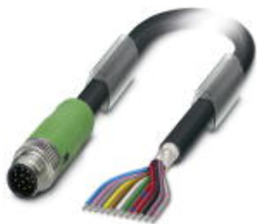
Sensor/Actuator cable, 12-position, PUR/PVC, Black RAL 9005, shielded, Plug straight M12 SPEEDCON, A-coded, on free cable end, Cable length: 3 m
