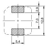
no sensitive traces underneath the component
