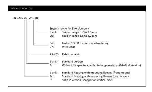
For example: FN 9255 MB-15-06 - FN 9255 dual stage IEC inlet with rear mount flanges, medical version, 15A rated current and fast-on terminals
