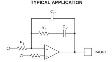
Figure 10. Current Loop Compensation
