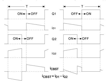
Figure 8. Timing Waveforms for Synchronization Scheme
