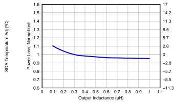
Figure 14. Normalized Power Loss vs Output Voltage Figure 15. Normalized Power Loss vs Output Inductance
