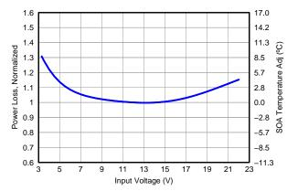
Figure 13. Normalized Power Loss vs Input Voltage
