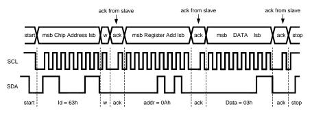
Figure 34. Write Cycle W = Write (SDA = "0") R = Read (SDA = "1") Ack = Acknowledge (SDA Pulled Down by Either Master or Slave) ID = Chip Address, 63h for LM3643
