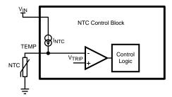
Figure 31. Temp Detection Diagram
