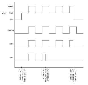
Figure 27. IR Mode with Boost
