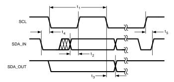
Figure 1. I<sup>2</sup>C-Compatible Interface Specifications
