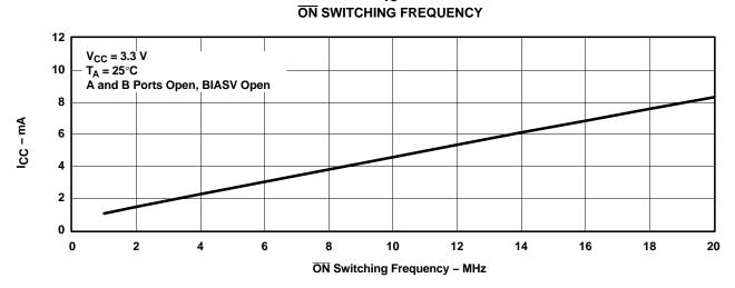
Figure 2. Typical I<sub>CC</sub> vs  $\overline{\text{ON}}$  Switching Frequency
