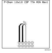
Typical  $R_{\theta JA} =$ 275°C/W when mounted on minimum
