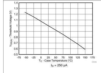
Figure 6. Threshold Voltage vs Temperature
