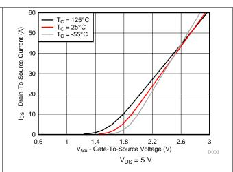
Figure 2. Saturation Characteristics
