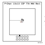
Typical  $R_{\theta JA} = 70^{\circ}C/W$  when mounted on 1 inch<sup>2</sup> of 2 oz. Cu.
