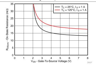
Figure 7. On-State Resistance vs Gate-to-Source Voltage
