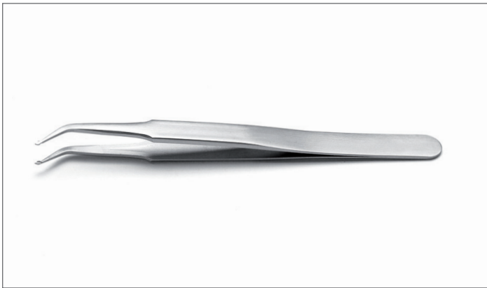
SM111.SA 4 3/4" 120 mm For holding and positioning 0.5-1 mm cylindrical devices; flat base grooved tips ( 2 mm long)
