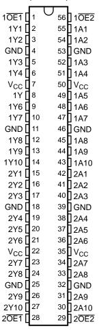
Active bus-hold circuitry holds unused or undriven inputs at a valid logic state. Use of pullup or pulldown resistors with the bus-hold circuitry is not recommended.
