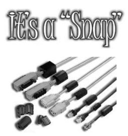
Fair-Rite announces a new series of snap on assemblies for round cables. The capsule shaped assemblies are both functional and ergonomic. Available in five sizes they will fit cables from 4mm to 12.7mm in diameter and provide impedance of 150 - 315 ohms @ 100 MHz. The housings are polypropylene with a flammability rating of UL94-V0. A kit containing parts in both 44 and newly developed 31 material, which extends useful range to below 25MHz is available.
