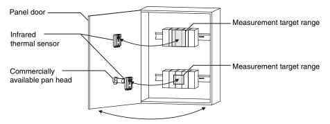
• Installing on the internal side surface of the panel by using a commercially available pan head
