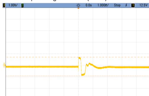
Output voltage waveform(0.71 KV)
