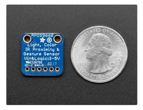
Since there are four IR sensors, you can measure the changes in light reflectance at each of the cardinal locations over time and turn those changes into gestures. Our interface library can detect directional gestures (left to right, right to left, up to down, down to up), but in theory more complicated gestures like zig-zag, clockwise or counterclockwise circle, near to far, etc. could also be detected with additional code.
