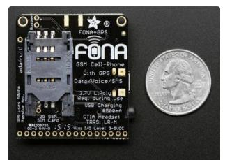
The SIM card holder is on the back. It holds a very-standard "Mini SIM" Micro SIMs will not work! Make sure you get a "Mini SIM"
