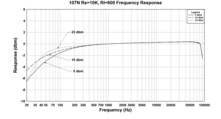
107N Rs=10K, RI=600 THD+N 107N Rs=10K, RI=600 Phase Shift 50 - 0 stors -- 10 stors -- 20 stors 23 dbm 40 60 10 dbm 0 dbm 30 40 23 dbm (%) N+OH1 Degrees 20 20 0 dbm 10 dbm 10 0 -20 Ó -10 -40 20 30 40 50 70 100 200 300 500 700 1000 2000 3000 5000 10000 20000 50000 100000 20 30 40 50 70 100 200 300 500 700 1000 2000 3000 5000 10000 20000 50000 100000 Frequency (Hz) Frequency (Hz)
