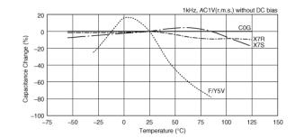
Capacitance - temperature characteristics
