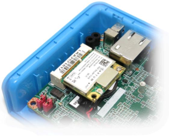
3. Connect the antenna pigtail to the U.FL *RF jack*.
