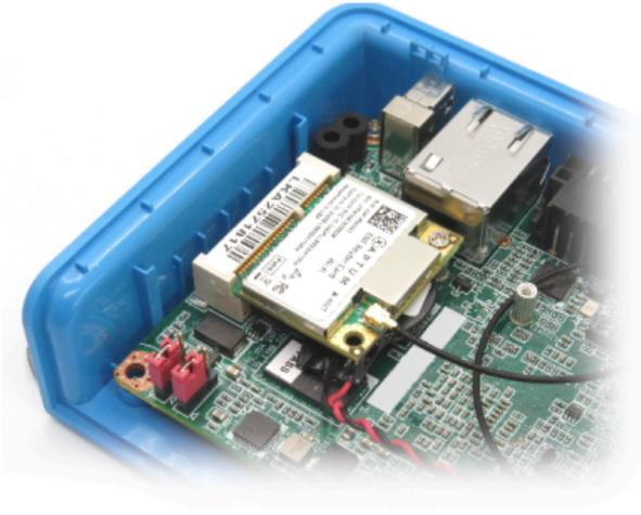
4. Connect an approved external antenna to the RP-SMA connector on the host device.
