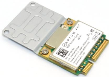
2. Insert the *router card* into the Mini PCIe slot on the host device, and secure according to the host device's instructions.
