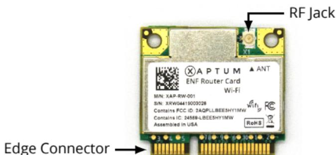
**Edge Connector** The Mini PCIe *edge connector* plugs into a Mini PCIe slot on the host. It provides power and a USB 2.0 connection to the router card.
