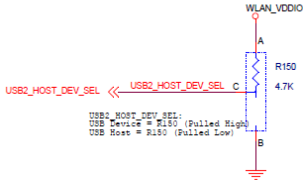
Figure 4-5. USB2_HOST_DEV_SEL Strapping Option
