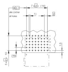
1) ø 0,6±0.05 Diameter of finished plated-through hole ø 0,7 ±0.02 Diameter of drilled hole
