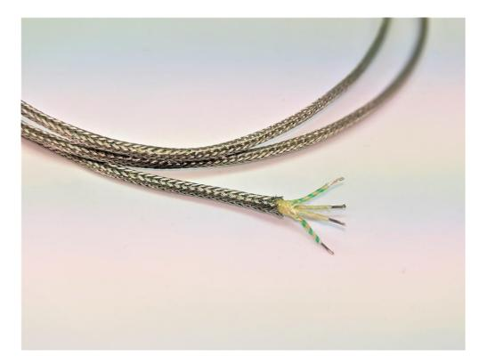
Glassfibre insulated flat pair construction, conductors laid flat, Glassfibre insulated with Glassfibre jacket, silicone varnished throughout + stainless steel overbraid for added protection and mechanical strength. Good temperature resistance but not suitable where fluids are present.
