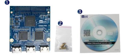
Figure 1-1 The HDMI-FMC package contents
