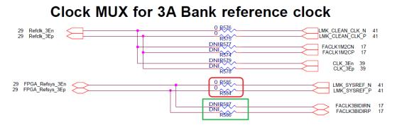
Figure 4-6 The resistors need to be reworked
