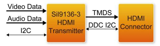
Figure 3-1 Sil9136-3 HDMI transmitter
