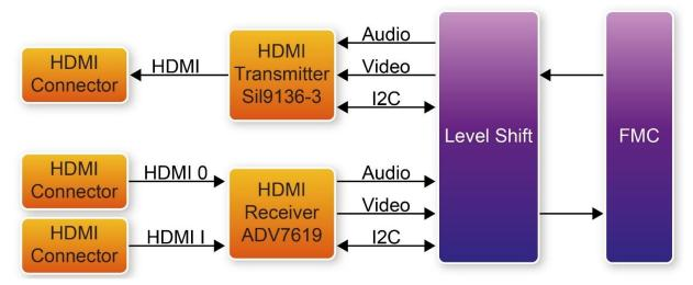
Figure 2-3 Block Diagram of the HDMI-FMC Board
