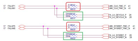
Figure 4-5 The resistors need to be reworked
