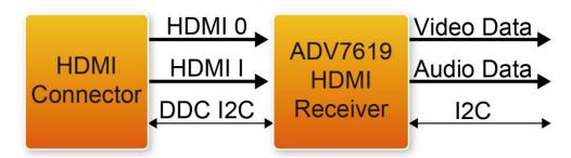
Figure 3-2 ADV7619 HDMI receiver
