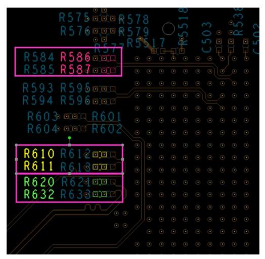
Figure 4-7 The resistors positions on the PCB
