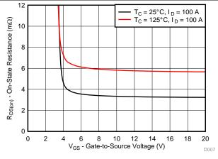
Figure 7. On-State Resistance vs Gate-to-Source Voltage
