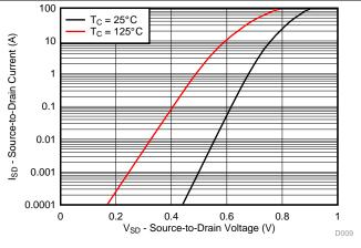
Figure 9. Typical Diode Forward Voltage
