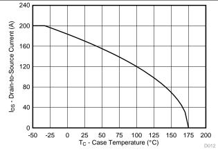
Figure 12. Maximum Drain Current vs Temperature
