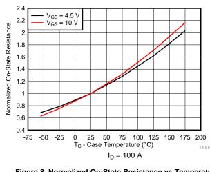
Figure 8. Normalized On-State Resistance vs Temperature
