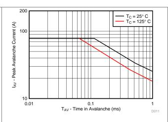
Figure 11. Single Pulse Unclamped Inductive Switching
