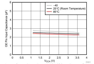
Figure 1. Input Capacitors for OE Pin (C<sub>I</sub>) vs Power Supply (V<sub>CCA</sub>)
