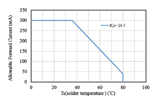
Fig 6. Forward Current Derating Curve
