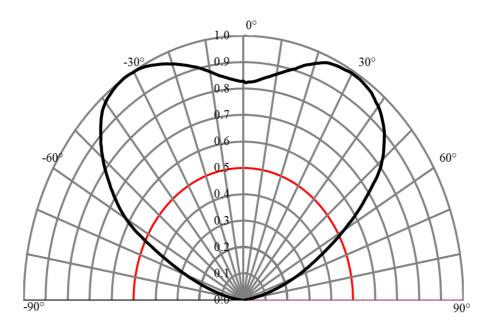
Fig 5. Radiation Characteristics
