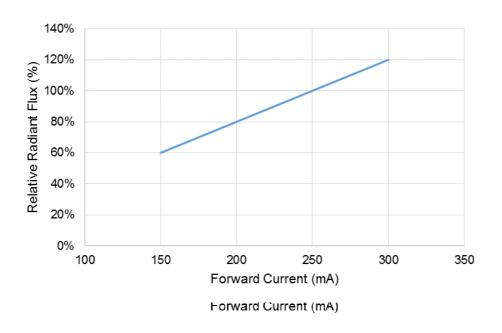
Fig 1. Relative Radiant Flux vs. Forward Current
