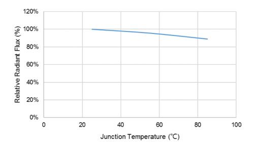
Fig.4 Relative Radiant Flux vs Junction Temperature
