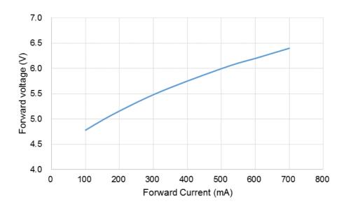
Fig 3. Forward Current vs. Forward Voltage
