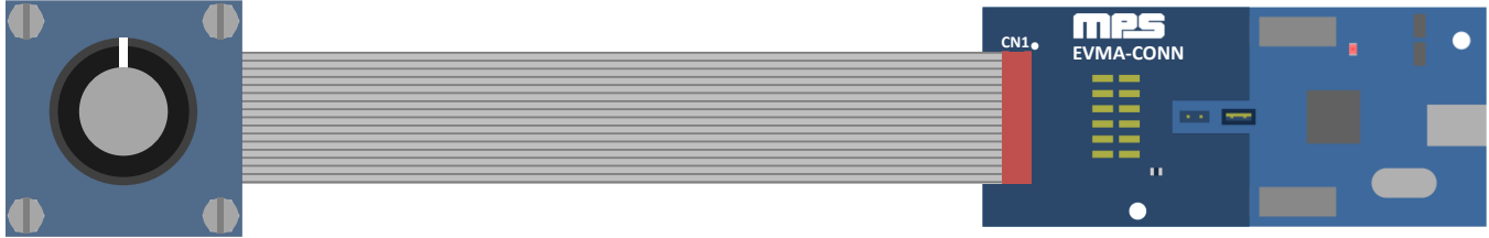
Figure 18: Connect EVKT-KNOB to EVMA-CONN Board (Top View)
