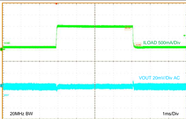
Figure 60. Load Transient V_{OUT} = 3.3\text{ V}
