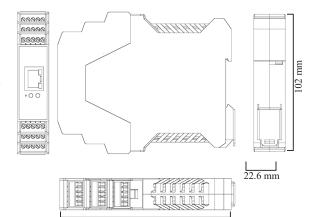
Screw Terminals 3.5mm pitch, #22 - #14, 0.5mm<sup>2</sup>-2.5mm<sup>2</sup> pin power supply
