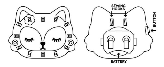
If the battery is already in your badge, then pull out the paper or plastic tab and your badge should come on. If the battery isn't already in, then push it all the way in to the battery holder, with the + side facing upwards (matching the + on the battery holder).
