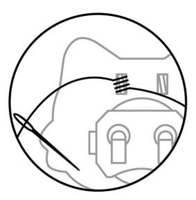
Anchor the thread again next to the hook to hold it tight, then run a stitch to where you'd like the sensor to be positioned.
