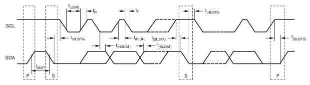
Figure 7. Two-Wire Timing Diagram
