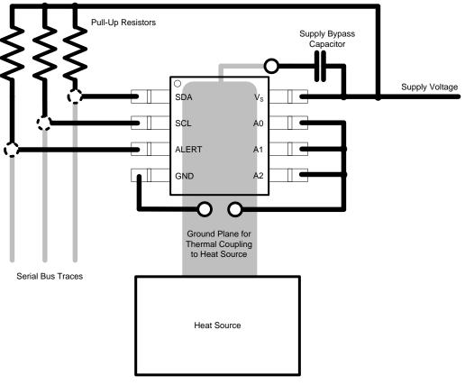
Figure 20. TMP275 Layout Example
