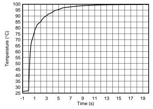
Figure 17. Temperature Step Response
