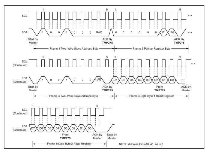
Figure 9. Two-Wire Timing Diagram for Read Word Format
