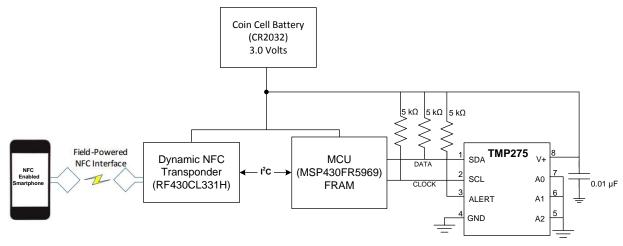
Figure 19. Temperature Data Logger
