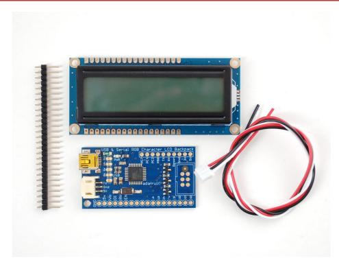
The backpack comes with a piece of header you can use to fit the display on. Its handy to have a solderless breadboard to attach the header on straight.
