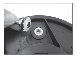
2.2 Place the washer on the air valve or plug, remove the backing film on the sealing material and install with the sealing material surface against the end plate.
