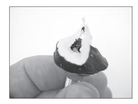
2.3 Torque the air valve or plug to 50-70 in-lbs (5.7 -8.1 kgm) and check for leaks.
