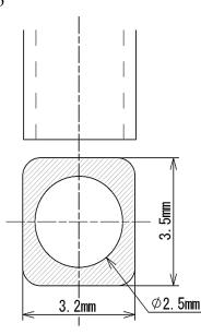
\*Nozzle with chamfering is recommended
