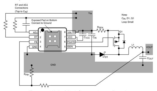
Figure 32. LM25085 Buck Converter Layout Example
