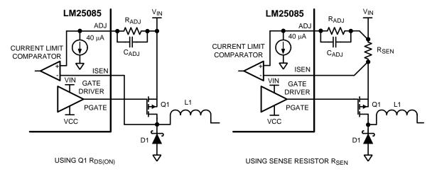
Figure 23. Current Limit Sensing
