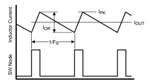
Figure 25. Inductor Current Waveform
