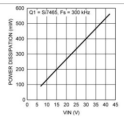
Figure 31. LM25085 Power Dissipation (Circuit Of Figure 32)
