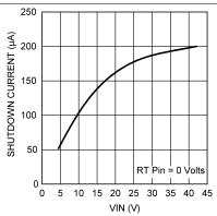
Figure 2. Input Operating Current vs.  $V_{\rm IN}$
