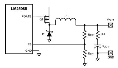
Figure 27. Lowest Cost Ripple Generating Configuration
