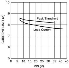
Figure 30. Current Limit vs. V<sub>IN</sub> (Circuit Of Figure 32)
