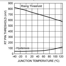
Figure 21. Rt Pin Shutdown Threshold vs. Temperature
