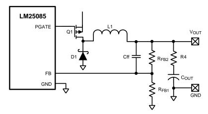
Figure 26. Reduced Ripple Configuration
