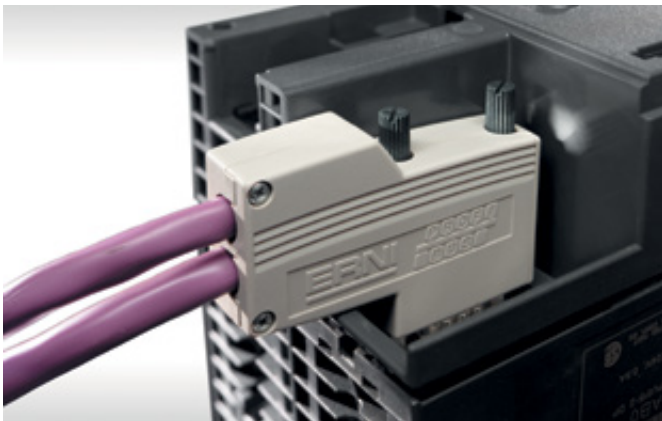
Integral T function, bus in, bus out
