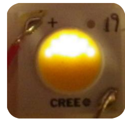
Figure 4: Partially illuminated CXA LED due to damaged bond wires
