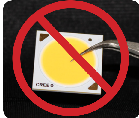
Figure 6: Correct and incorrect handling of CXA LED with fingers and tweezers
