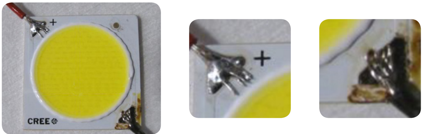
Figure 7: Left: Wires improperly attached to CXA LED, center: wires should not protrude beyond solder pads, right: excessive solder flux should be cleaned
