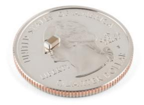
4.7  $\mu$ F capacitor on a quarter for size comparison.
