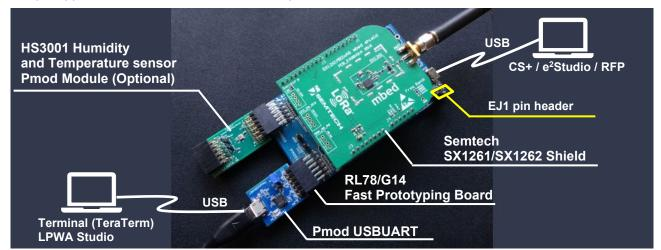
NOTE1: For Flash Programming or Debugging with IDE(CS+/e<sup>2</sup>studio), EJ1 pin header should be OPEN.
