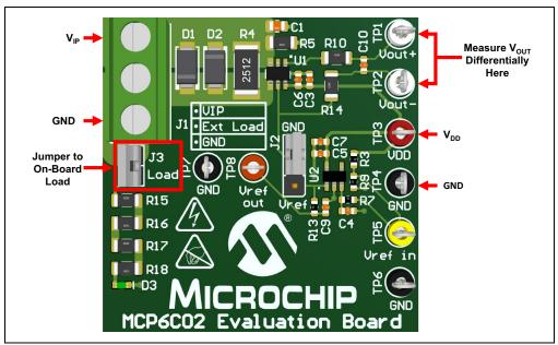
FIGURE 2-5: Using the On-Board Load.
