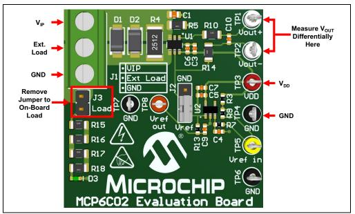
FIGURE 2-6: Using the External Load.
