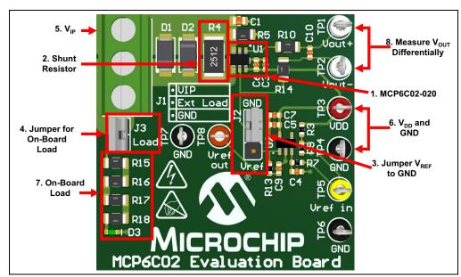
FIGURE 2-3: Out-of-the-Box Setup.
