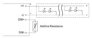
"DO NOT connect "DIM- to -V"
