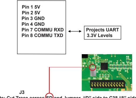
Note: Cut Trace across SD and Jumper "D" side to C38 "8" side GND to take the RS232 Tranceiver out of circuit.
