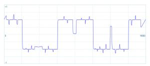
Also included is a fully programmable arbitrary waveform generator with a 8 k-sample buffer.
