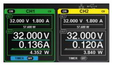
The T3PS3000 Display is 4.3 inch (10.92 cm) color TFT-LCD, with 5 Digits Voltage with 1 mV Resolution and 4 Digits Current with 1 mA resolution.
